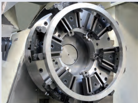
For clamping thin walled workpieces
